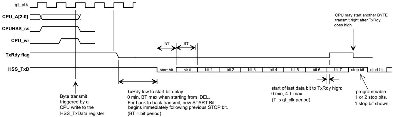
qt\_clk, CPU\_A, CPUHSS\_cs, CPU\_wr are internal signals, included in the diagram to illustrate the relationship between CPU operations and HSS port operations.
