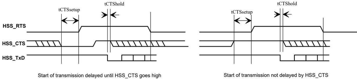
t<sub>CTSsetup</sub>: HSS\_CTS setup time before HSS\_RTS = 1.5T min.
