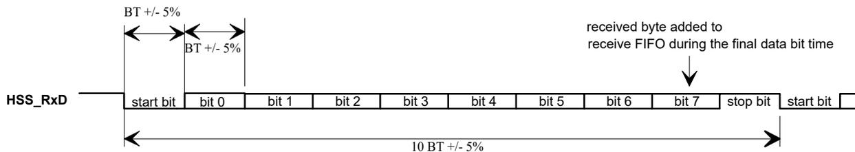
Receive data arrives asynchronously relative to the internal clock. Incoming data bit rate may deviate from the programmed baud rate clock by as much as  $\pm 5\%$  (with HSS\_RATE value of 23 or higher).
