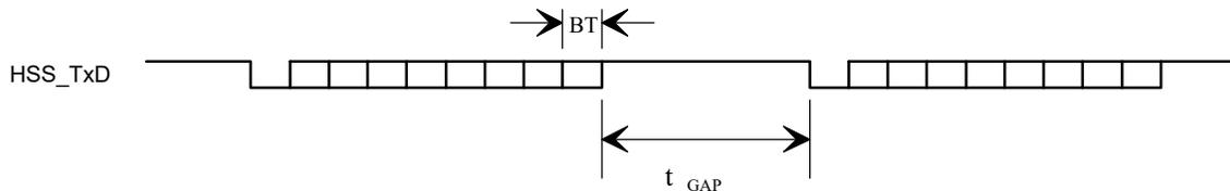
BLOCK mode transmit timing is similar to BYTE mode, except the STOP bit time is controlled by the HSS\_GAP value.
