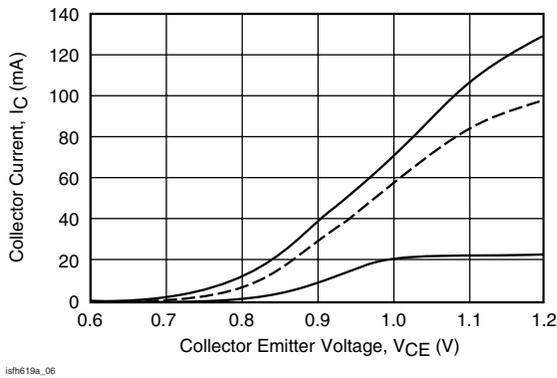
Fig. 5 - Collector Current vs. Collector Emitter Voltage
