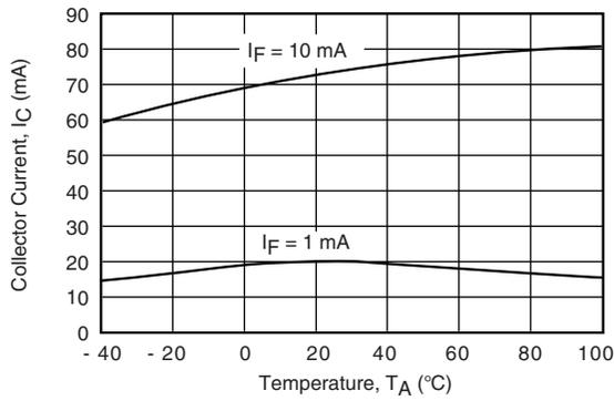
Fig. 4 - Collector Current vs. Ambient Temperature
