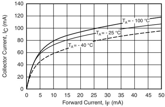
Fig. 3 - Collector Current vs. Forward Current
