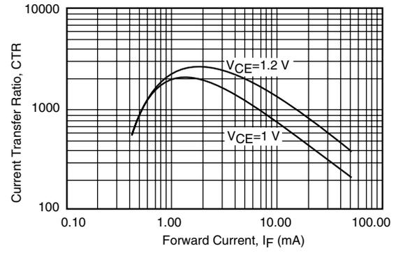
Fig. 7 - Current Transfer Ratio vs. Forward Current
