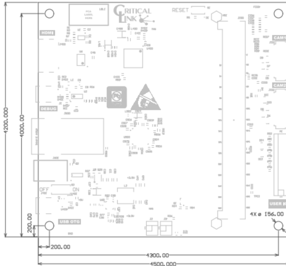
Figure 2: MitySOM-5CSX VDK Baseboard, Mounting Hole Locations (Top View)
