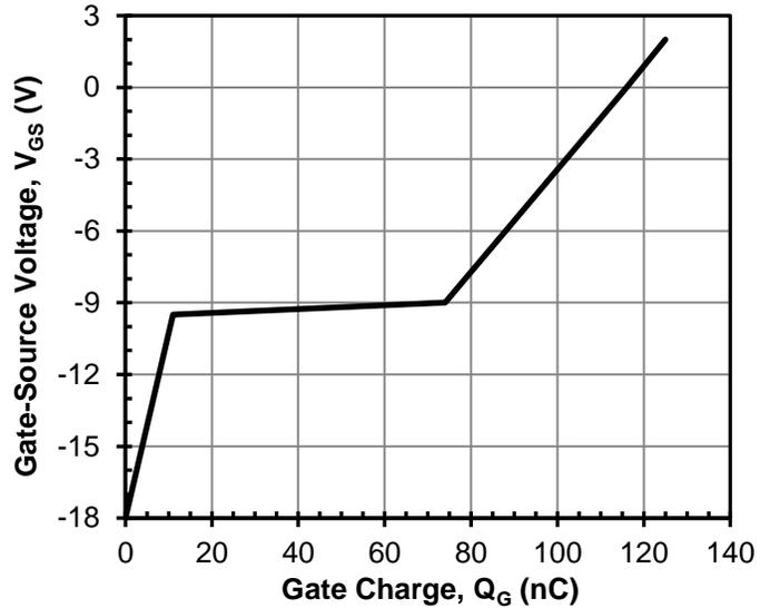
**Figure 16** Typical gate charge
