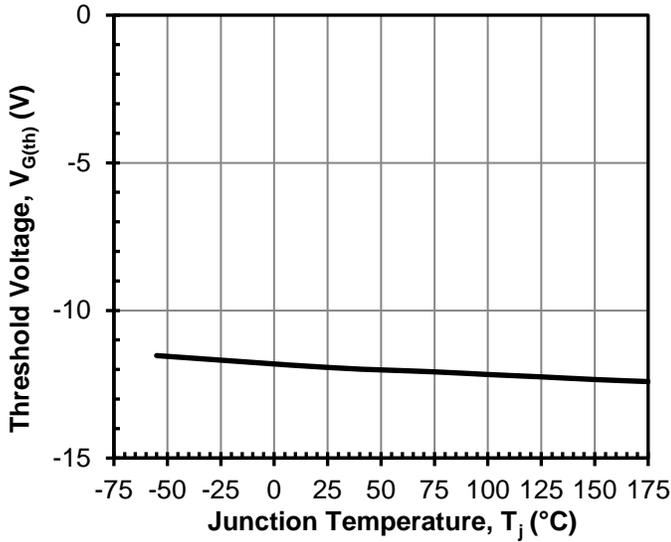
**Figure 9** Threshold voltage vs.  $T_j$
