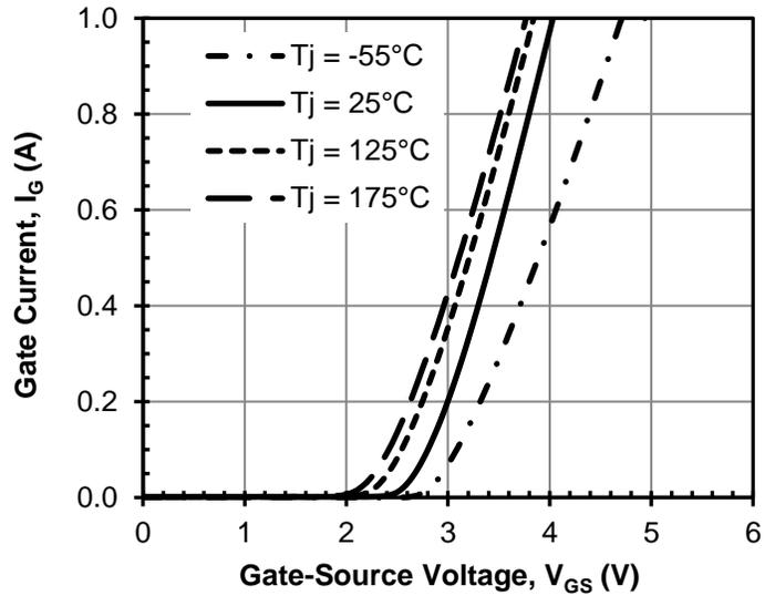
**Figure 14** Typical gate forward current
