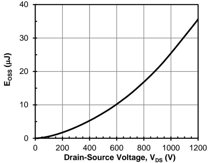
**Figure 10** Typical stored energy in  $C_{OSS}$
