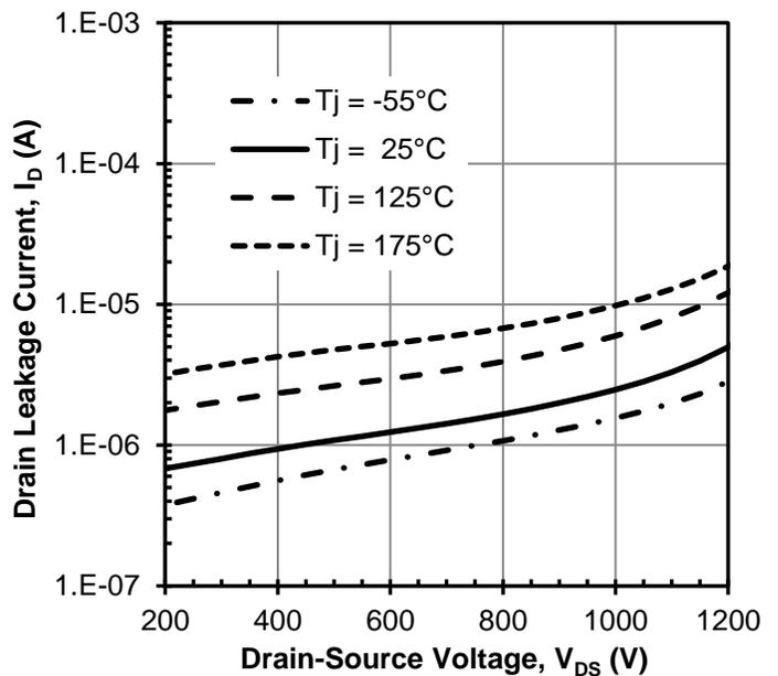
**Figure 4 Typical drain-source leakage**
