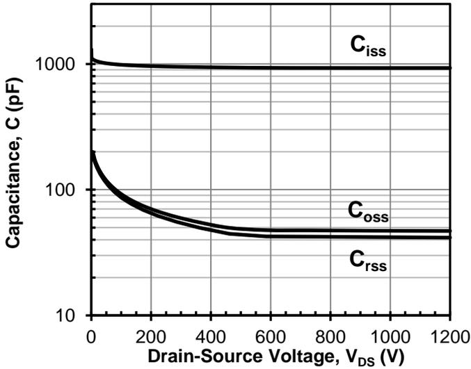
**Figure 5** Typical capacitances at 100kHz and  $V_{GS} = -20V$
