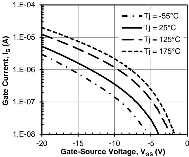
**Figure 13** Typical gate leakage current
