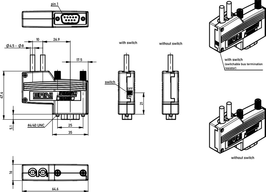
ERbic Profibus with PU interface, vertical
