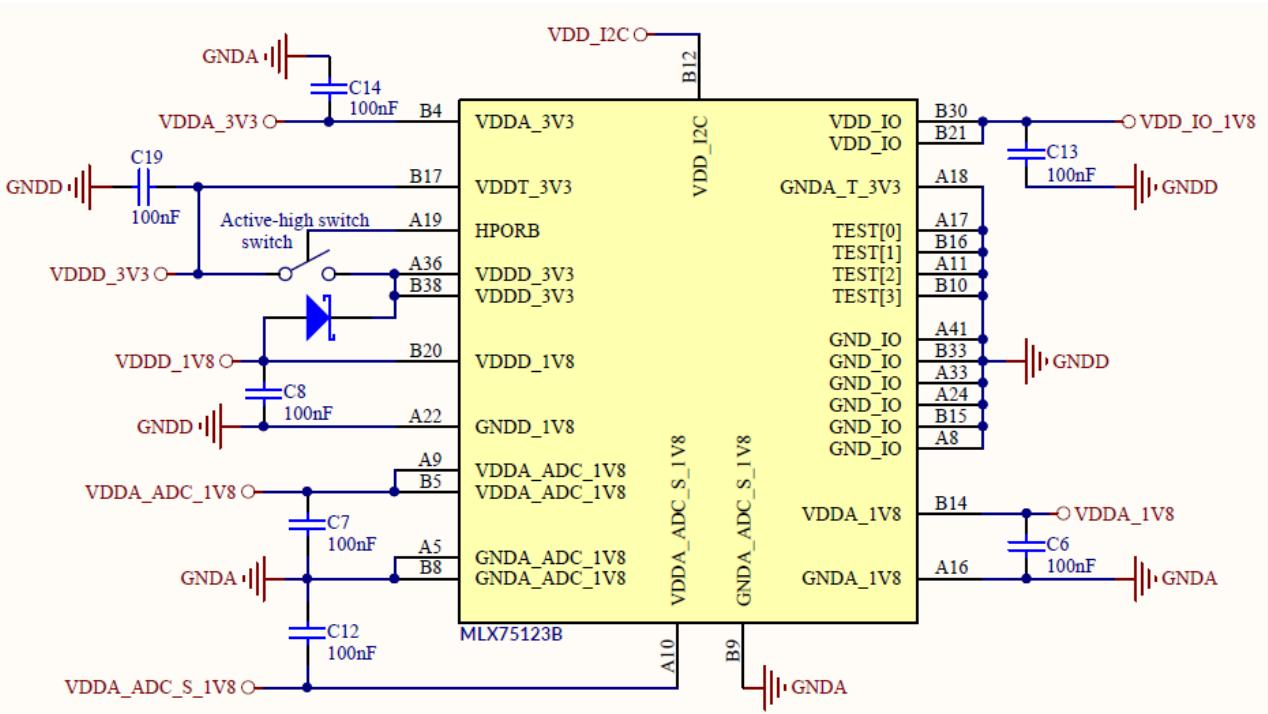
*Figure 6: HPORB signal recommended implementation.*
