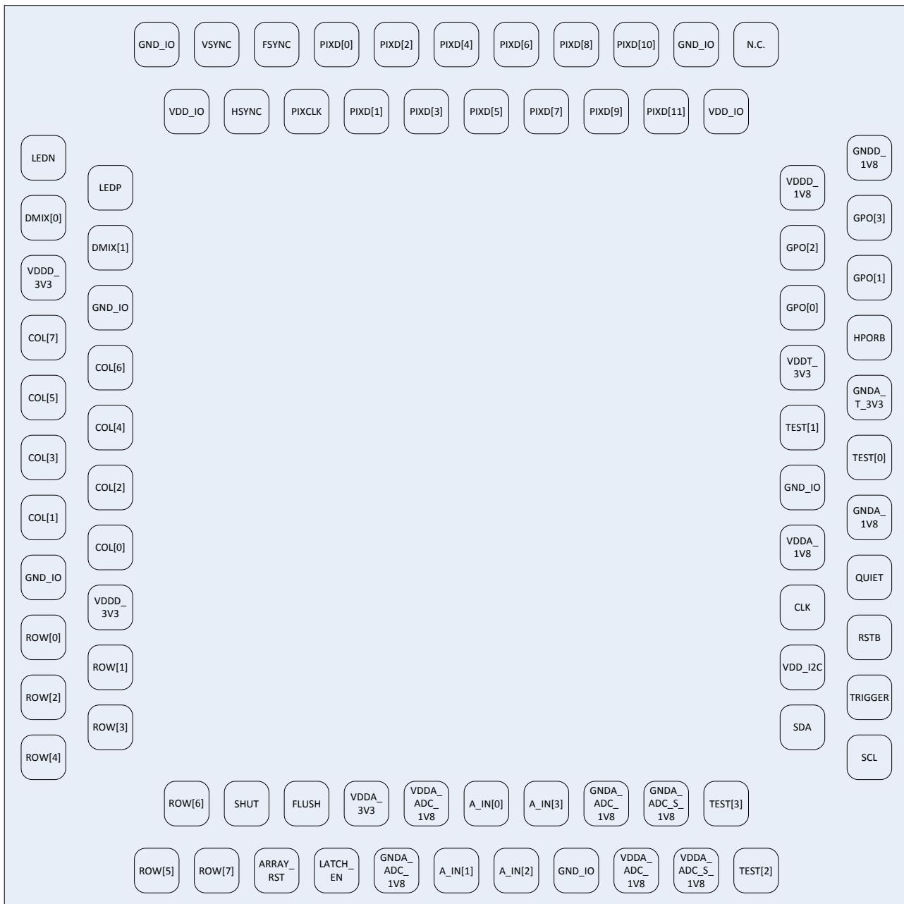
Figure 4: Array QFN package, 84 pins. Top view.
