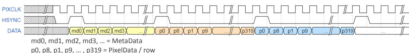
During a phase the maximum # of rows is limited to 251, depending on the features that are enabled or disabled.
