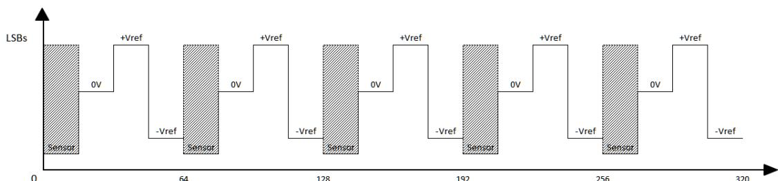
Figure 8 : EN\_TEST\_ADC row for Mode #4 (12bit A)
