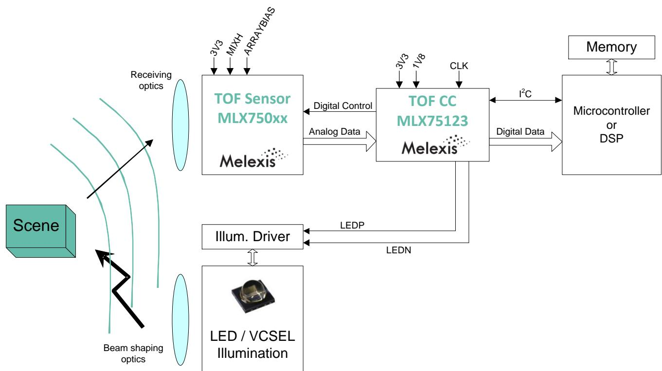
Figure 2: System architecture
