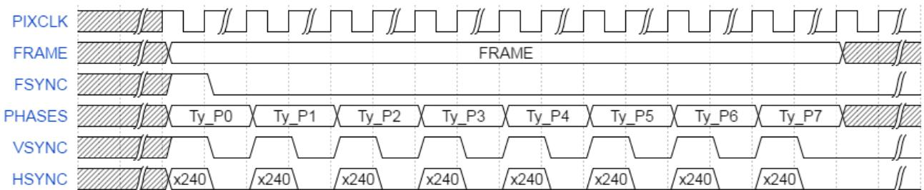
Figure 7 : FSYNC, VSYNC & HSYNC timing diagram<sup>1</sup>
