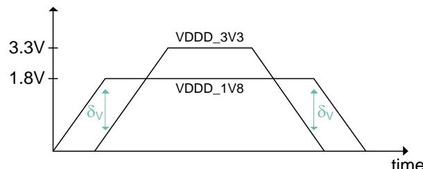
Figure 5 : Voltage domains startup sequence
