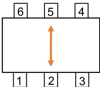
The arrow represent the axis of sensitivity of the two sensors inside the device (as referenced as Rout in Figure 1) that have their axis of sensitivity 180 degrees out of phase with each other.
