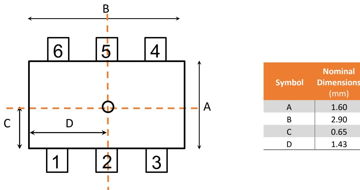
**Figure 3: Axis of Sensitivity**
