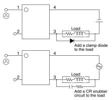
2) Even if spike voltages generated at the load are limited with a clamp diode if the circuit wires are long, spike voltages will occur by inductance. Keep wires as short as possible to minimize inductance. • Check the connection diagrams in the catalog and be sure to connect the terminals correctly.
