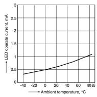
7. LED turn off current vs. ambient temperature characteristics Load voltage: 10V (DC);
