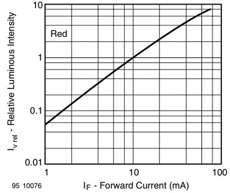
Figure 5. Relative Luminous Intensity vs. Forward Current
