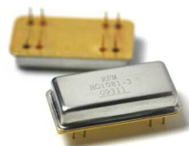
DIP16-8 Case 25.02 mm x 12.83 mm x 6.35 mm
