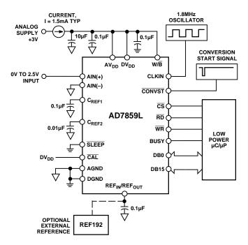
Figure 23. Typical Low Power Circuit
