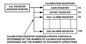
Figure 5. Calibration Register Arrangement
