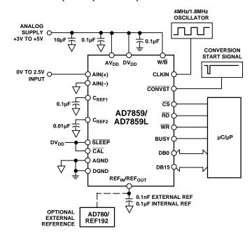
Figure 8. Typical Circuit
