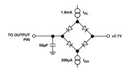
Figure 1. Load Circuit for Digital Output Timing Specifications
