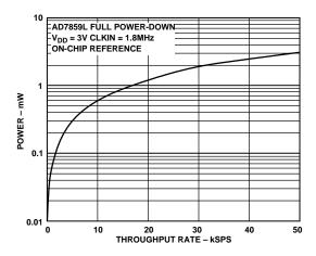
Figure 27. Power vs. Throughput AD7859L
