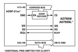
Figure 38. AD7859/AD7859L to ADSP-21xx Parallel Interface
