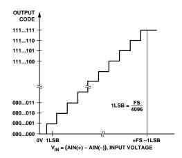
Figure 14. AD7859/AD7859L Unipolar Transfer Characteristic
