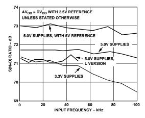
Figure 19. SNR vs. Frequency
