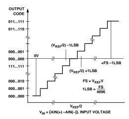
Figure 15. AD7859/AD7859L Bipolar Transfer Characteristic
