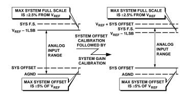
Figure 32. System (Gain + Offset) Calibration
