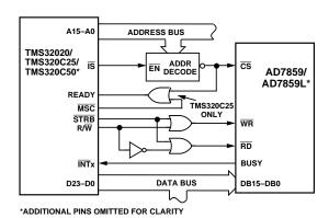
Figure 39. AD7859/AD7859L to TMS32020/C25/C5x Parallel Interface
