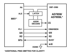
Figure 42. AD7859/AD7859L to 8051 Parallel Interface
