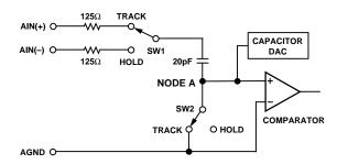
Figure 9. Analog Input Equivalent Circuit
