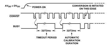
Figure 28. Timing Arrangement for Autocalibration on Power-On
