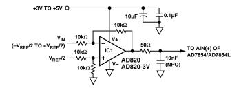
Figure 11. Analog Input Buffering
