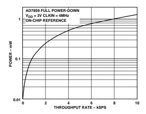
Figure 24. Power vs. Throughput AD7859
