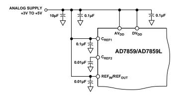
Figure 17. Relevant Connections,  $AV_{DD}$  as the Reference
