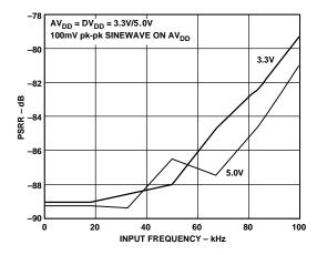
Figure 20. PSRR vs. Frequency
