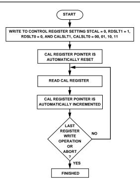
Figure 7. Flowchart for Reading from the Calibration Registers
