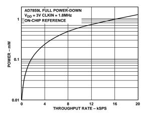
Figure 25. Power vs. Throughput AD7859L
