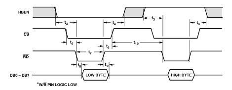
Figure 36. Read Cycle Timing for Byte Mode Operation
