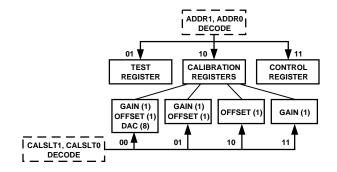
Figure 2. Write Register Hierarchy/Address Decoding
