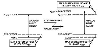
Figure 30. System Offset Calibration
