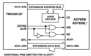
Figure 40. AD7859/AD7859L to TMS320C30 Parallel Interface AD7859/AD7859L to DSP5600x
