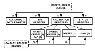
Figure 3. Read Register Hierarchy/Address Decoding
