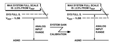
Figure 31. System Gain Calibration
