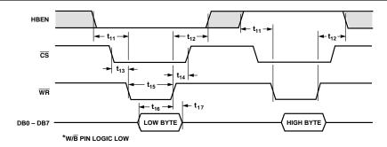
Figure 37. Write Cycle Timing for Byte Mode Operation
