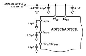
Figure 16. Relevant Connections Using Internal Reference
