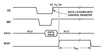
Figure 29. Timing Diagram for Full Self-Calibration
