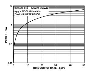
Figure 26. Power vs. Throughput AD7859
