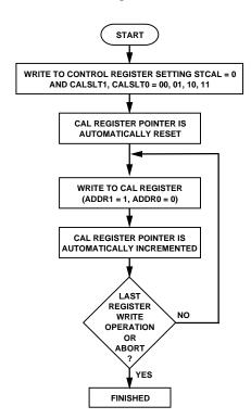
Figure 6. Flowchart for Writing to the Calibration Registers
