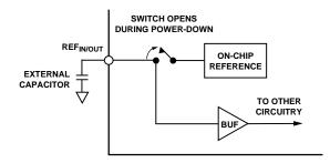
Figure 22. On-Chip Reference During Power-Down
