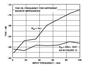
Figure 10. THD vs. Analog Input Frequency
