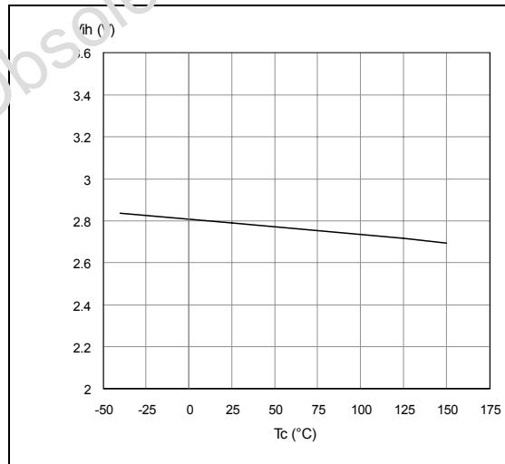
**Figure 18. Input low level**
