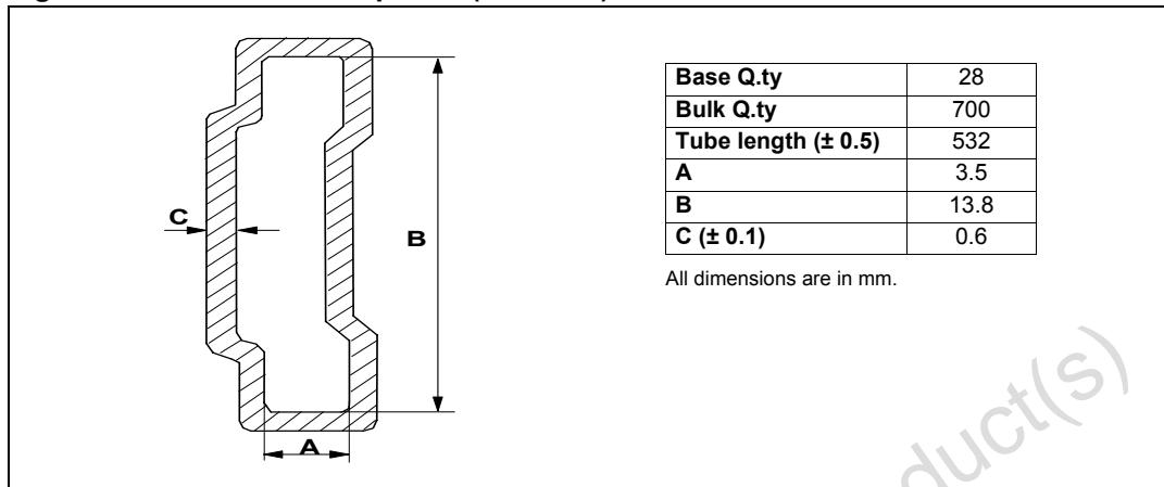
Figure 34. SO-28 tape and reel shipment (suffix "13TR")
