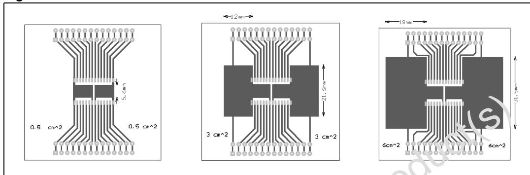
Note: Layout condition of  $R_{th}$  and  $Z_{th}$  measurements (PCB FR4 area : 58 mm x 58 mm, PCB thickness = 2 mm, Cu thickness = 35  $\mu$ m, Copper areas: 0.5  $cm^2$ , 3  $cm^2$ , 6  $cm^2$ ).
