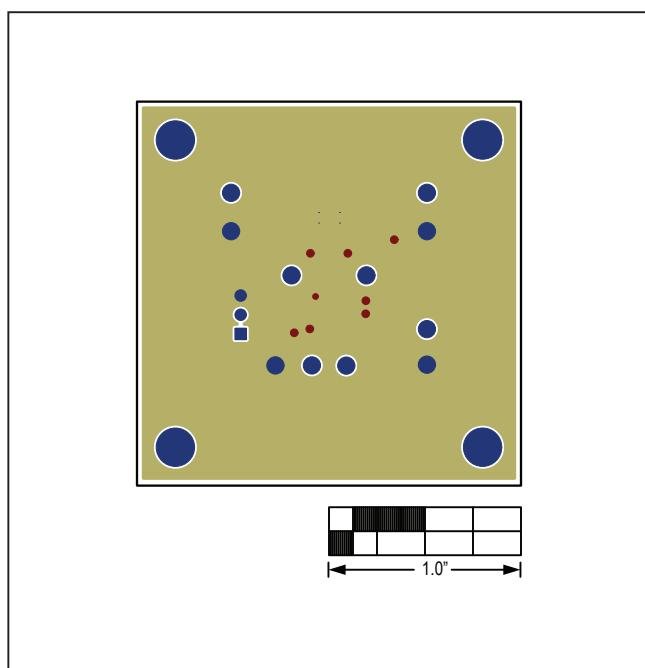
Figure 4. MAX44284 EV Kit PCB Layout—Solder Side
