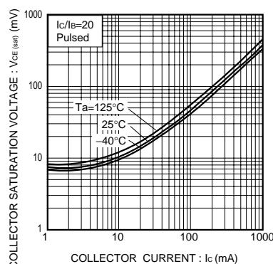
Fig.4 Collector-emitter saturation voltage vs. collector current (II)
