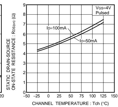
Fig.14 Static drain-source on-state resistance vs. channel temperature
