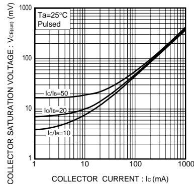
Fig.3 Collector-emitter saturation voltage vs. collector current (I)
