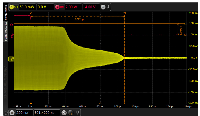
Figure 15. Switching Time [Insertion Loss to Isolation State]
