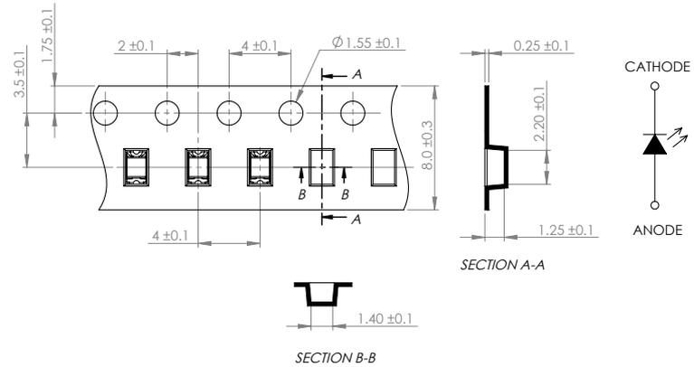
\*UNLESS OTHERWISE SPECIFIED TOLERANCES PER DECIMAL PRECISION ARE: X=±1 (±0.039), X.X=±0.5 (±0.020), X.XX=±0.25 (±0.010), X.XXX=±0.127 (±0.005). LEAD SIZE=±0.05 (±0.002), LEAD LENGTH=±0.75 (±0.030), MIN=<sup>+0.00</sup>/<sub>-0.00</sub> DECIMAL PRECISION, MAX=<sup>+0.00</sup>/<sub>-0.00</sub> DECIMAL PRECISION
