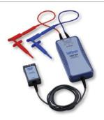
Low cost active differential probes are intended for measuring higher voltages. The differential techniques employed permit measurements to be taken at two points in a circuit without reference to the ground, allowing the oscilloscope to be safely grounded without the use of opto-isolators or isolating transformers.
