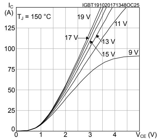
**Figure 5. IGBT transfer characteristics
