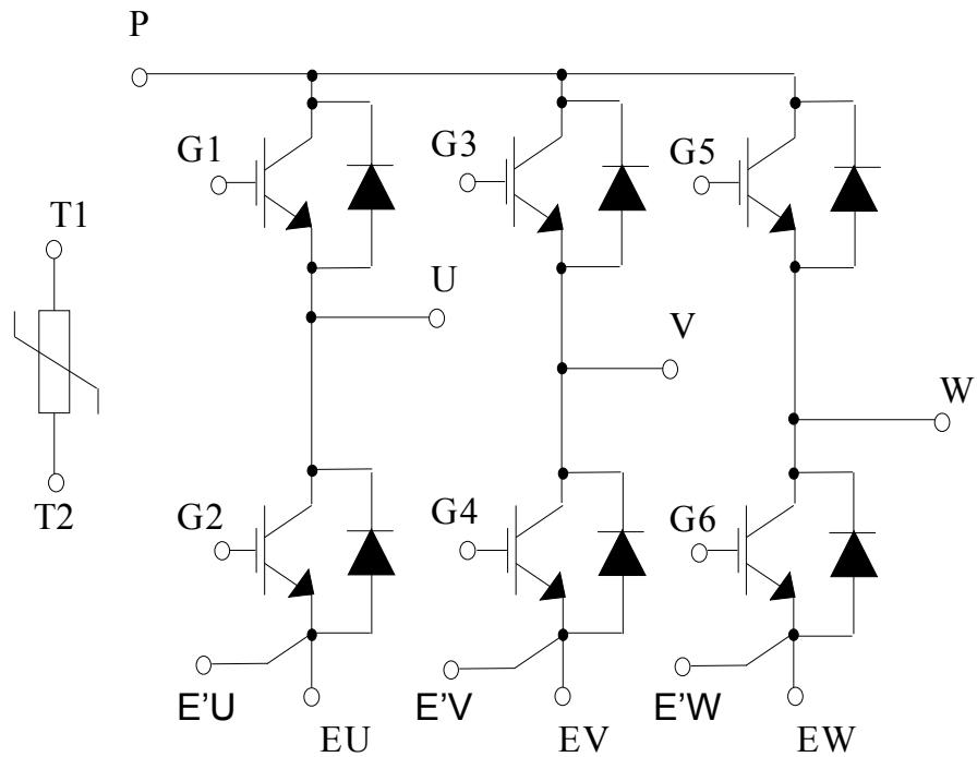
Figure 20. Package top view with sixpack pinout
