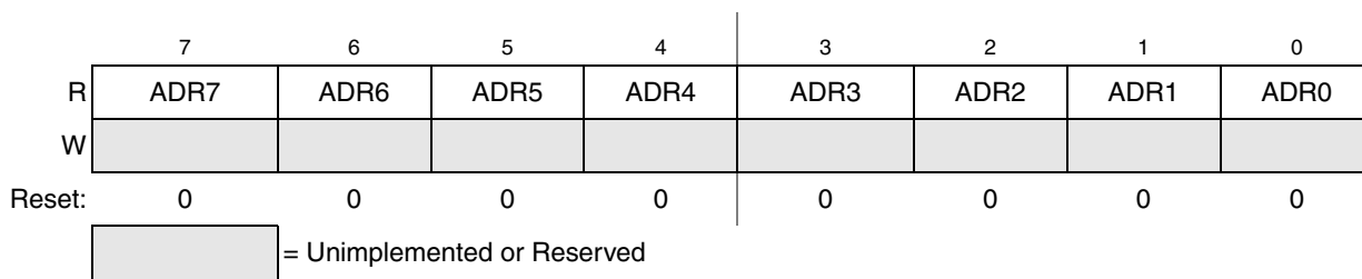
Figure 8-7. Data Result Low Register (ADCRL)
