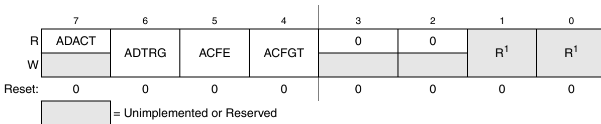
Figure 8-5. Status and Control Register 2 (ADCSC2)
