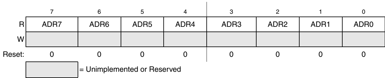
Figure 8-7. Data Result Low Register (ADCRL)
