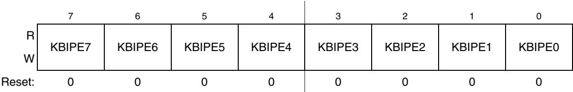
Figure 10-4. KBI Pin Enable Register
