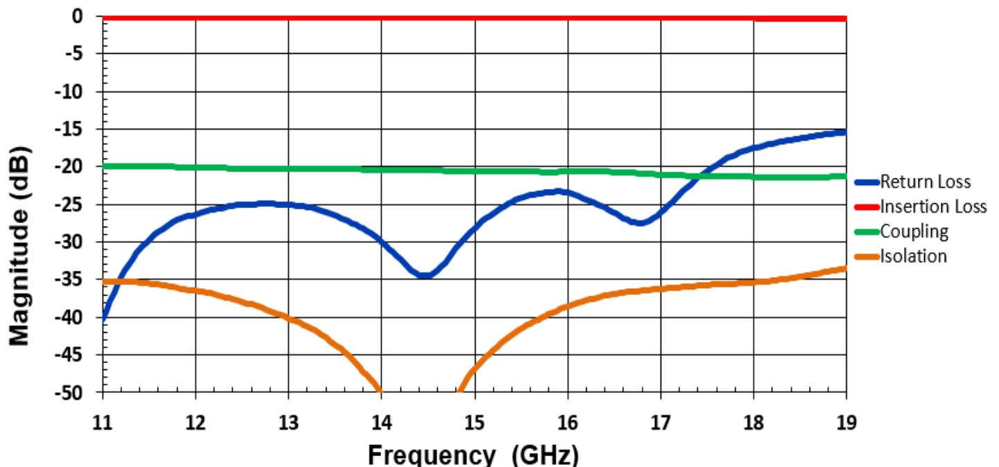
\*Typical measured performance mounted on RO4350B test board at 25°C.
