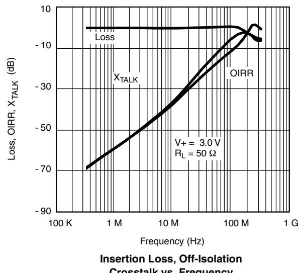
**Insertion Loss, Off-isolation Crosstalk vs. Frequency**
