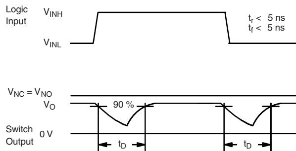
Figure 2. Break-Before-Make Interval
