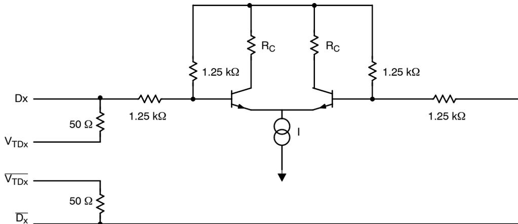
**Figure 6. Input Structure**
