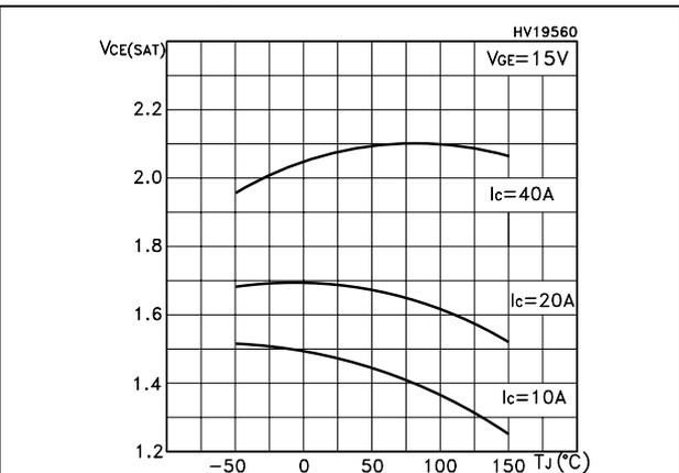
Figure 6. Collector-emitter on voltage vs collector current
