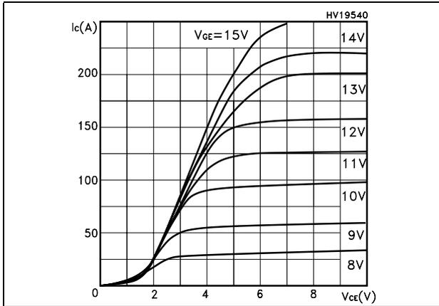
Figure 3. Transfer characteristics
