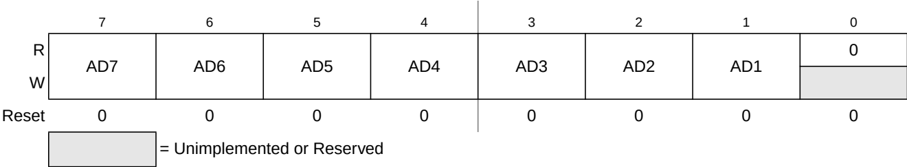
Figure 10-3. IIC Address Register (IICA)
