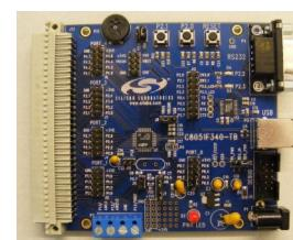
The Silicon Labs C8051F340-TB provides the microprocessor control and USB interfacing for the Development Kit. As a part of the Kit, no firmware changes are needed.
