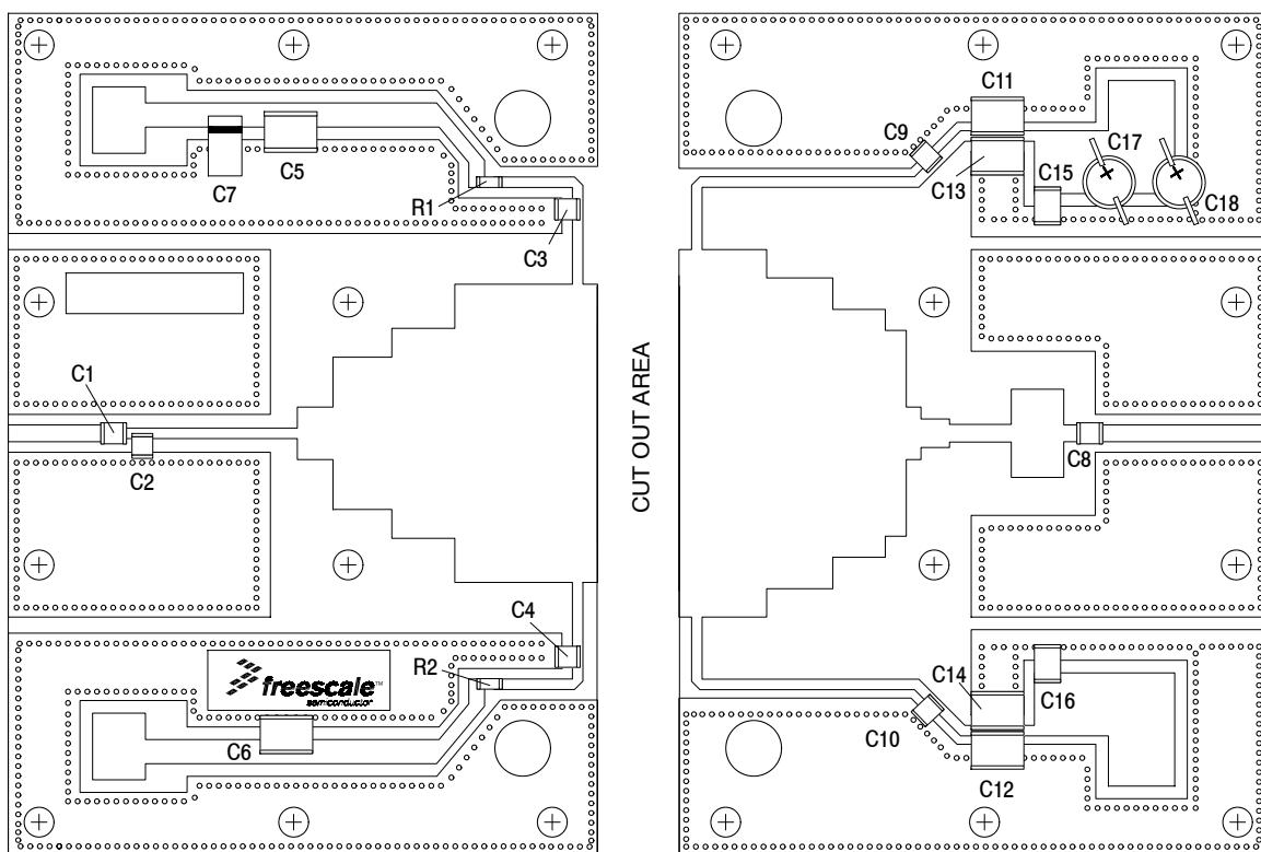
**Figure 13. MMRF1009HR5(HSR5) Test Circuit Component Layout — 960-1215 MHz**
