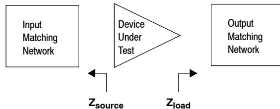
**Figure 12. Series Equivalent Source and Load Impedance**
