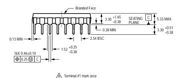
For Reference Only; not for tooling use (reference MS-001BB) Dimensions in millimeters
