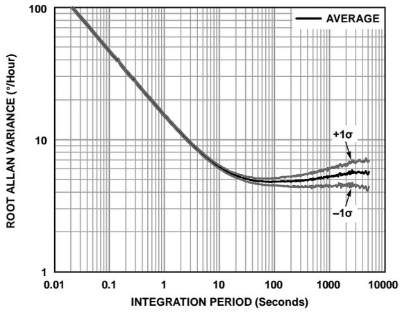
Figure 7. Gyroscope Allan Variance,  $T_c = 25^\circ\text{C}$
