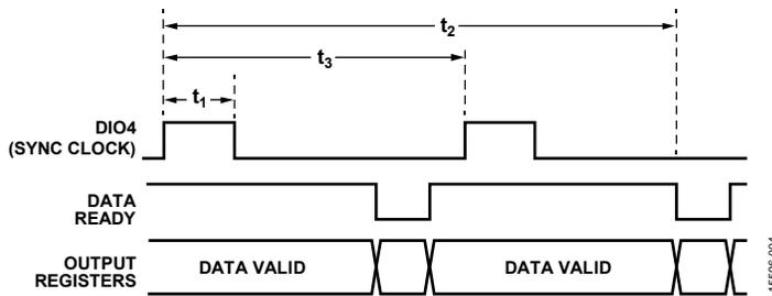
Figure 4. Input Clock Timing Diagram, FNCTIO\_CTRL[7:4] = 0xFD
