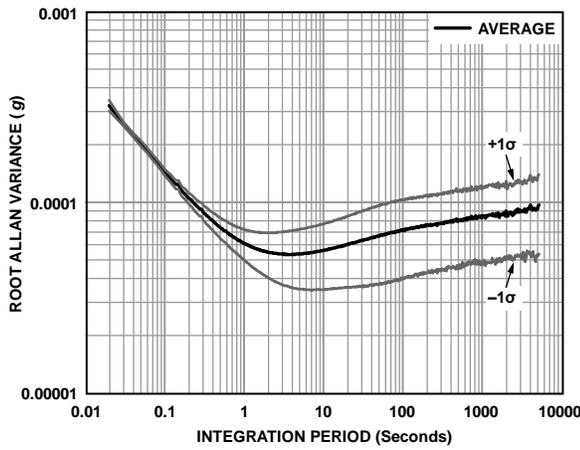
Figure 8. Accelerometer Allan Variance,  $T_c = 25^\circ\text{C}$
