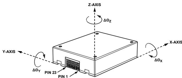
Figure 23. Delta Angle Axis and Polarity Assignments
