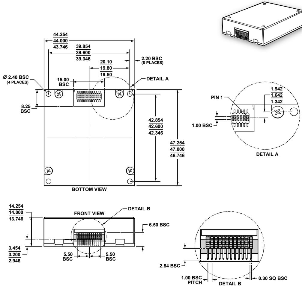
Figure 40. 24-Lead Module with Connector Interface [MODULE]
