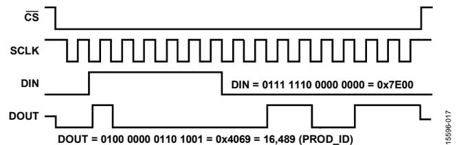
Figure 17. SPI Read Example, Second 16-Bit Sequence
