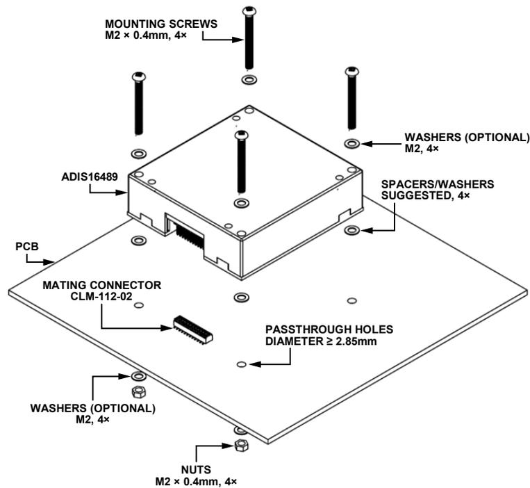
Figure 35. Mounting Example
