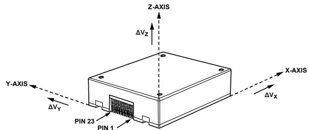
Figure 25. Delta Velocity Axis and Polarity Assignments
