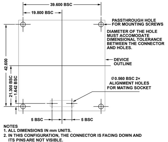
Figure 36. Suggested PCB Layout Pattern, Connector Down
