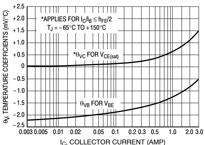
**Figure 12. Temperature Coefficients**
