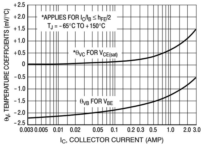
Figure 12. Temperature Coefficients
