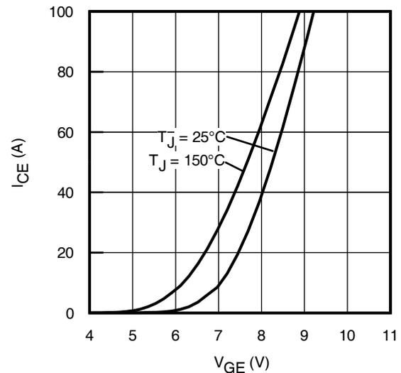
**Fig. 12 - Typ. Transfer Characteristics**
