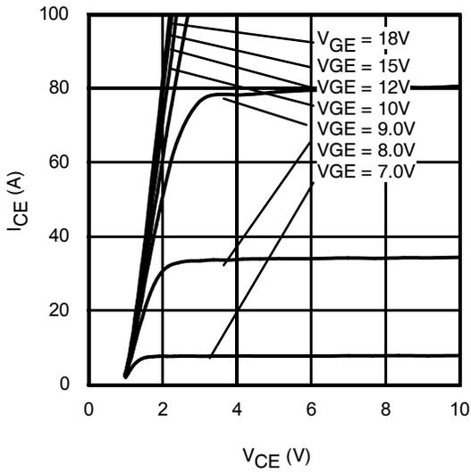
**Fig. 7 - Typ. IGBT Output Characteristics**
