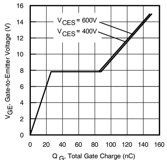
**Fig. 18 - Typical Gate Charge vs.  $V_{GE}$**
