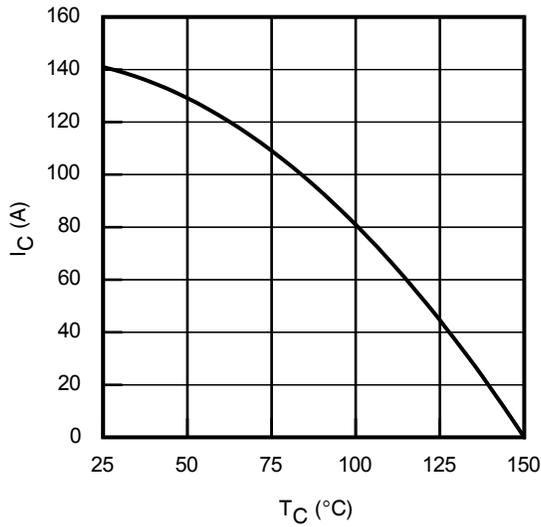
**Fig. 1 - Maximum DC Collector Current vs. Case Temperature**
