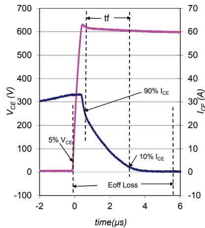
**Fig. WF1 - Typ. Turn-off Loss Waveform
