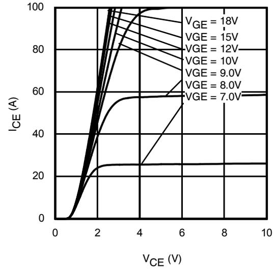
**Fig. 8 - Typ. IGBT Output Characteristics**
