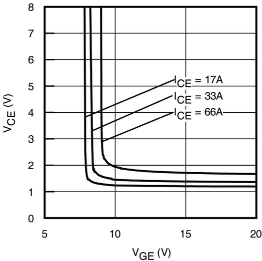
**Fig. 9 - Typical  $V_{CE}$  vs.  $V_{GE}$**
