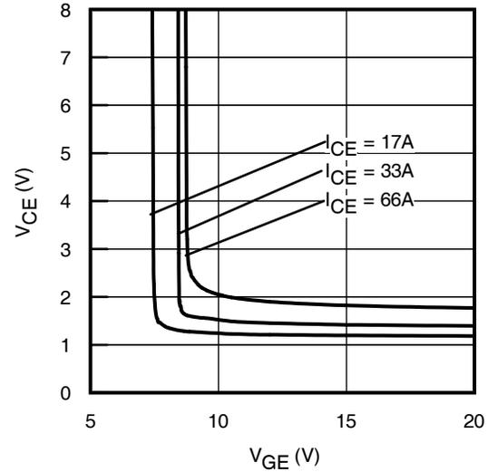
**Fig. 10 - Typical  $V_{CE}$  vs.  $V_{GE}$**
