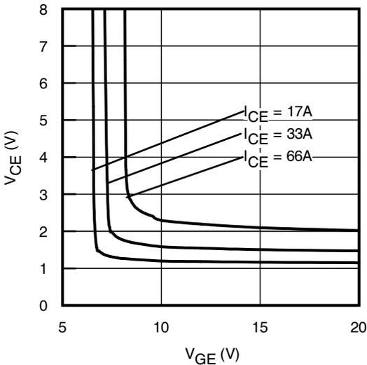
**Fig. 11 - Typical  $V_{CE}$  vs.  $V_{GE}$**
