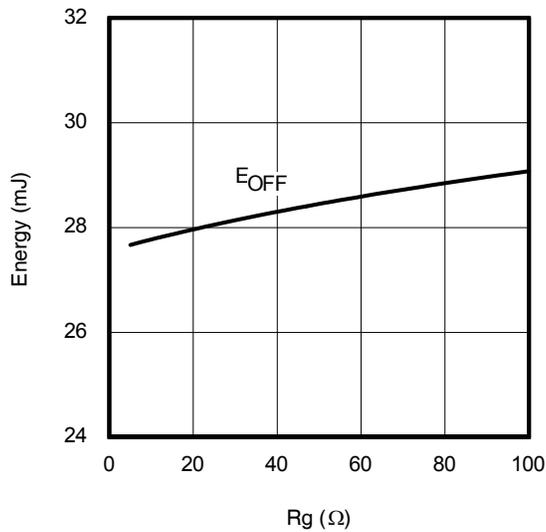
**Fig. 15 - Typ. Energy Loss vs.  $R_G$**
