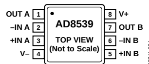
Figure 4. 8-Lead MSOP (RM-8)
