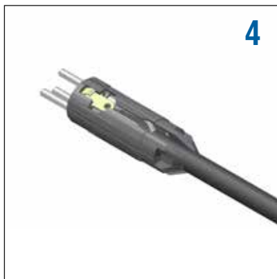
Install the cable clamp flush to the insert making sure to align the slot with the ground contact.
