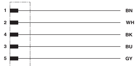
Contact assignment of the M12 plug and the M12 socket
