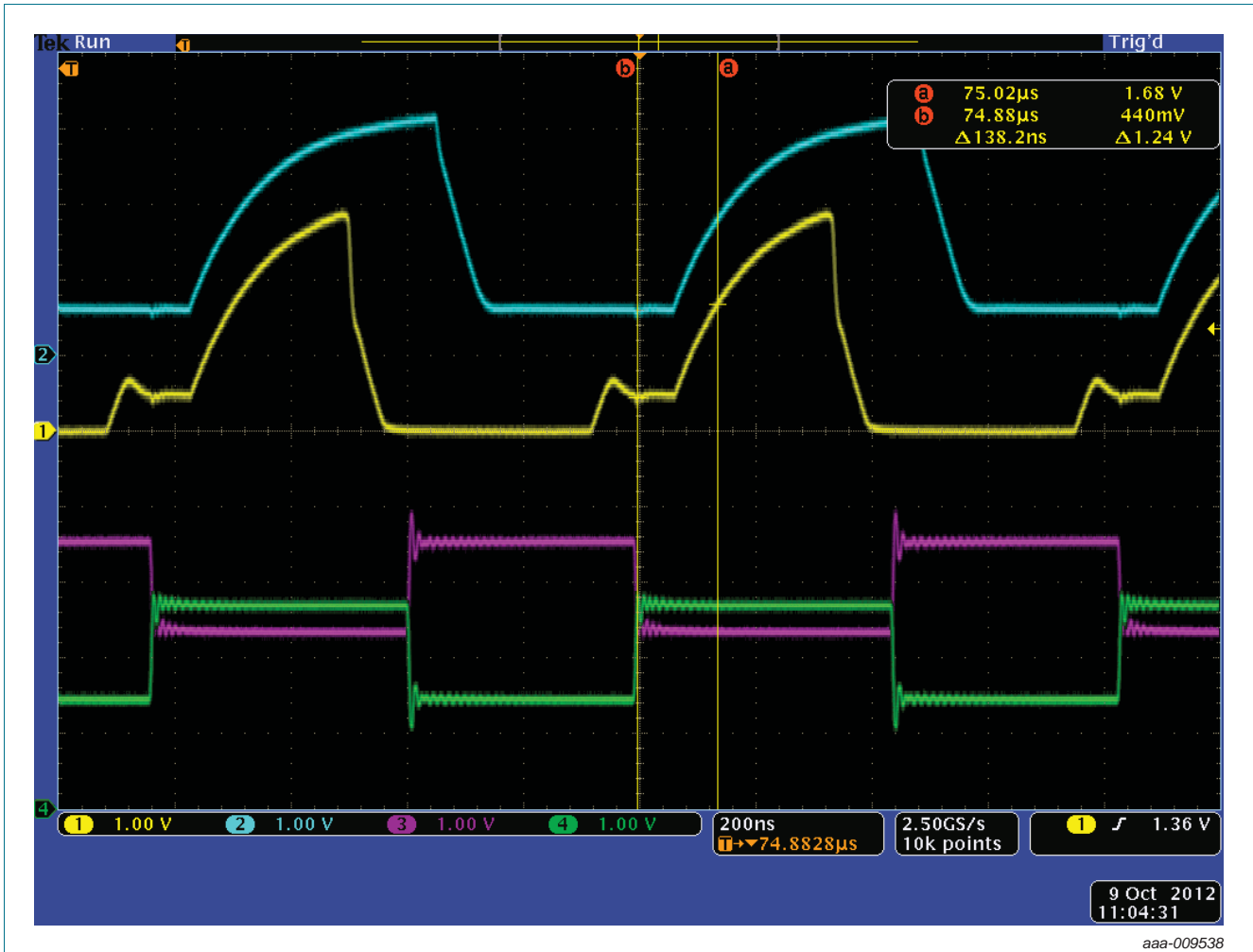
Fig 11. Differential bus waveform
