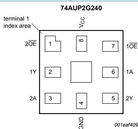
Fig. 5. Pin configuration SOT902-2 (XQFN8)
