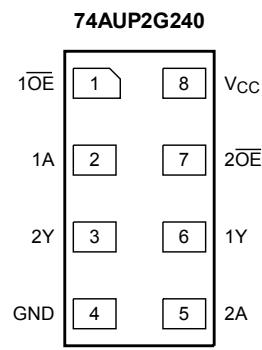
Fig. 4. Pin configuration SOT833-1, SOT1089, SOT1116 and SOT1203 (XSON8)
