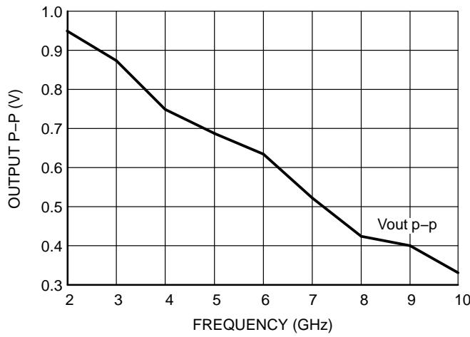
Figure 2. Typical  $V_{OUTP-P}$  vs. Frequency at  $25^\circ\text{C}$
