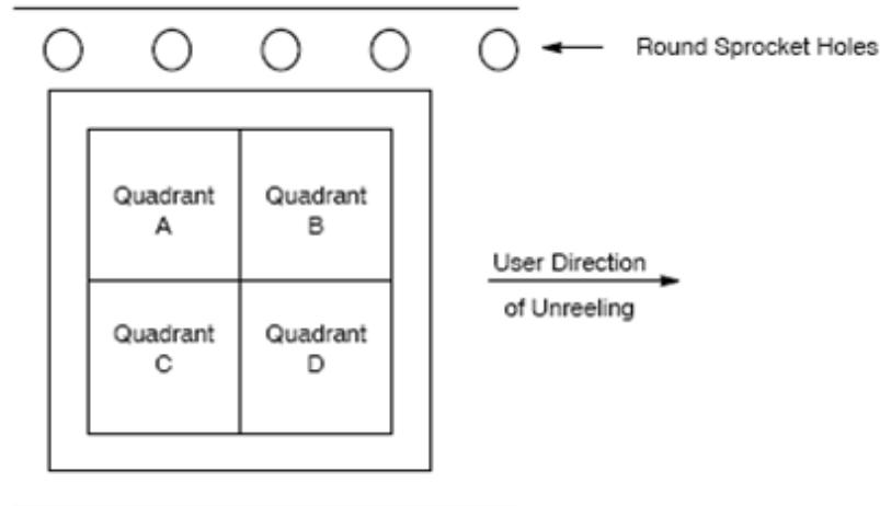
**Figure 17. Tape and Reel Pin 1 Quadrant Orientation**
