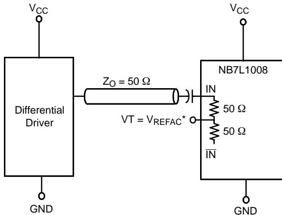
Figure 16. Capacitor-Coupled Single-Ended Interface
