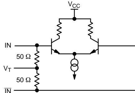
Figure 3. Input Structure
