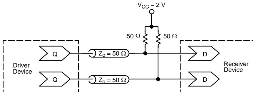
Figure 11. Typical Termination for Output Driver and Device Evaluation
