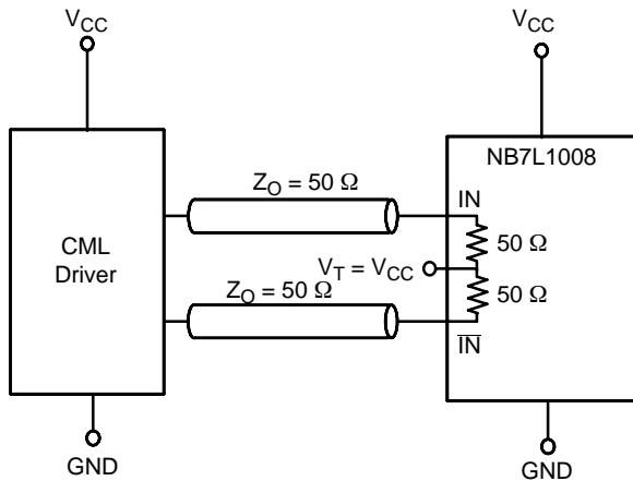
Figure 14. Standard 50 Ω Load CML Interface
