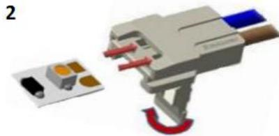
**2** - Insert LED flex ribbon, paying attention to ensure same polarity with wires. Notice that the LED should be aligned with the notched area of the connector and connector latch is on the bottom.
