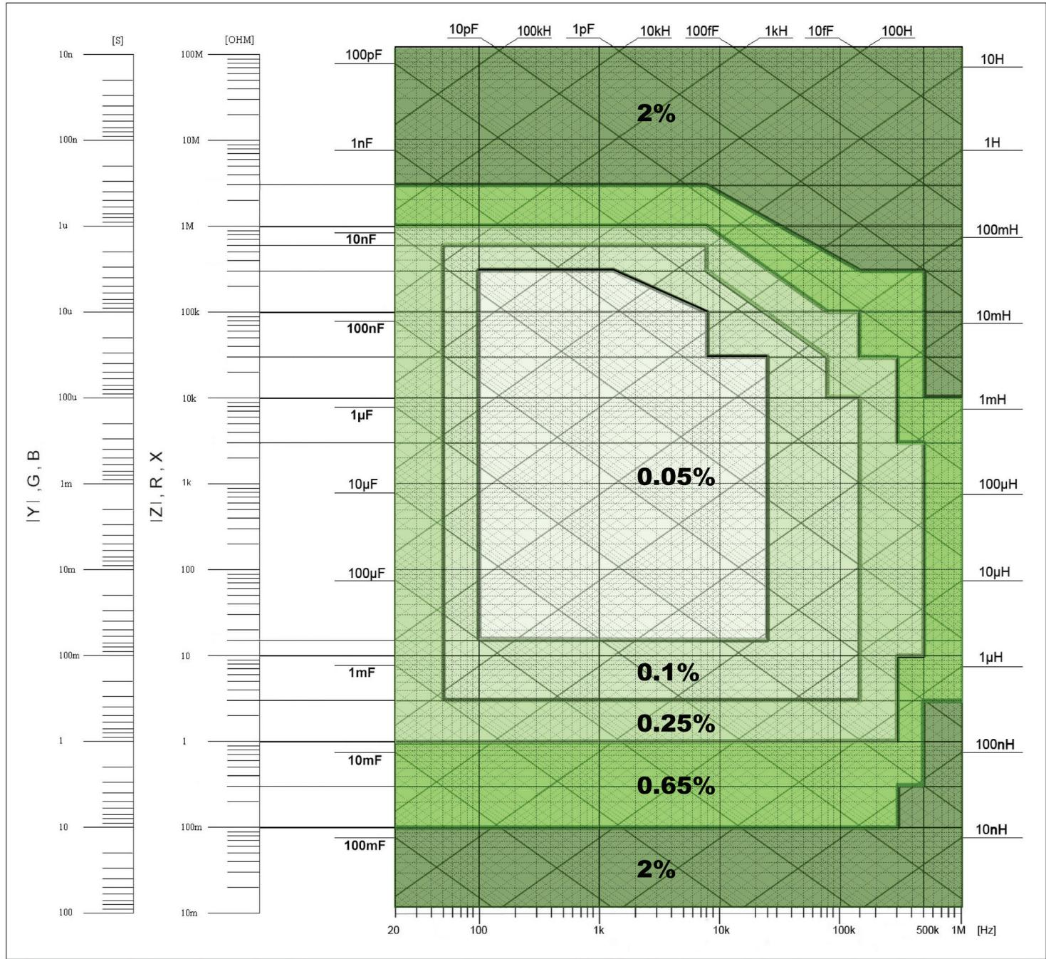
**DCR Accuracy:**  $A(I + Rx / 5 M\Omega + 16 m\Omega / Rx)|\%| \pm 0.2 m\Omega$   $A=0.25$  for slow & medium speed,  $A=0.5$  for fast speed
