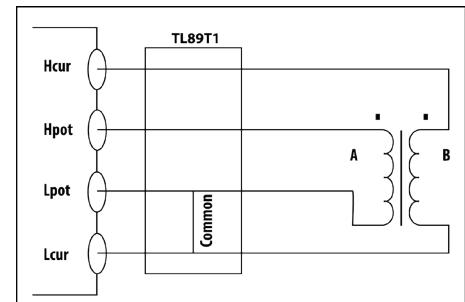
Diagram showing the TL89T1 connected to a transformer under test.
