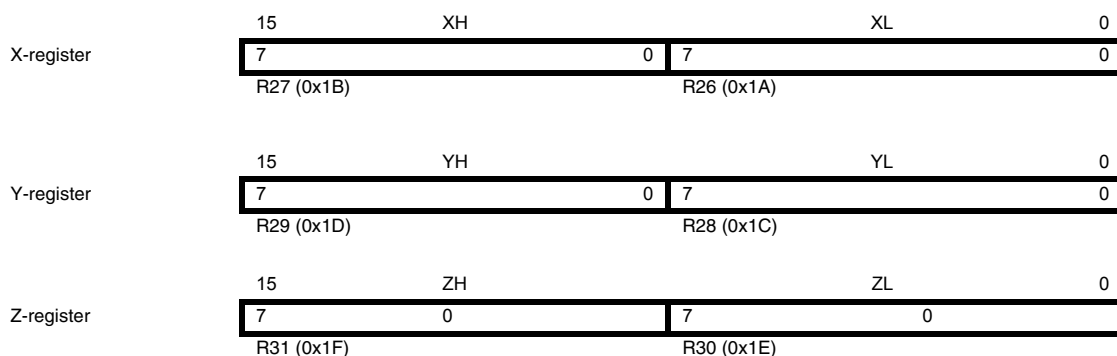
Figure 5-3. The X-, Y-, and Z-registers.
