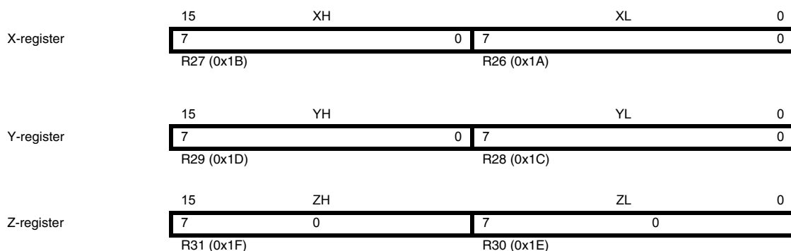
Figure 5-3. The X-, Y-, and Z-registers.
