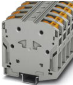
High-current terminal block, Connection method: Push-in connection, Cross section: 25 mm 2 - 95 mm 2 , AWG: 4 - 3/0, Width: 25 mm, Color: gray, Mounting type: NS 35/15
