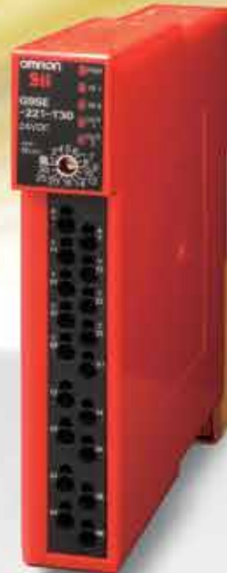
2 safety outputs with OFF-delay G9SE-221-T05/T30
