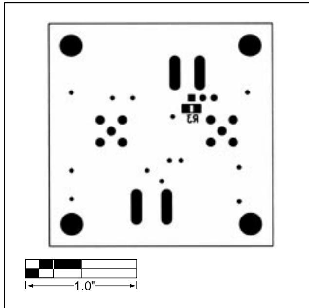
Figure 3. MAX4213 EV Kit Component Placement Guide—
