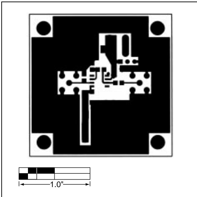
Figure 4. MAX4213 EV Kit PC Board Layout—Component Side
