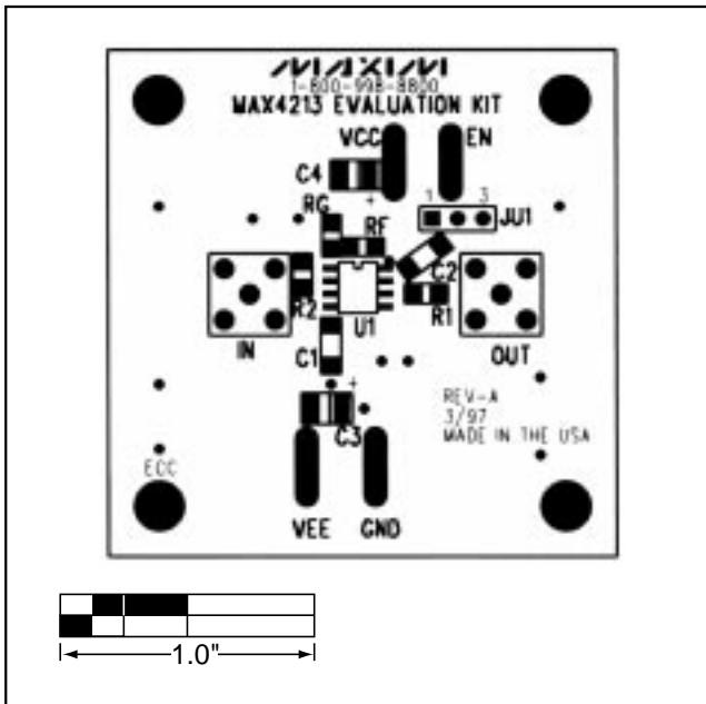
Figure 2. MAX4213 EV Kit Component Placement Guide—
