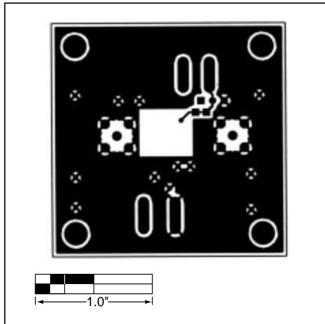
Figure 5. MAX4213 EV Kit PC Board Layout—Solder Side
