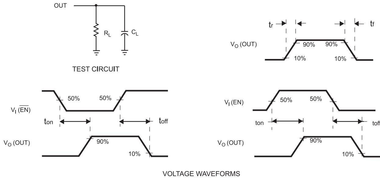
Figure 1 — Definition of Tr, Tf, Ton and Toff
