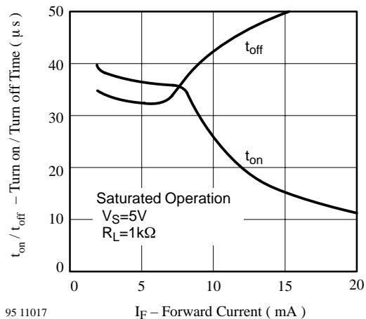
Figure 16. Turn on / off Time vs. Forward Current
