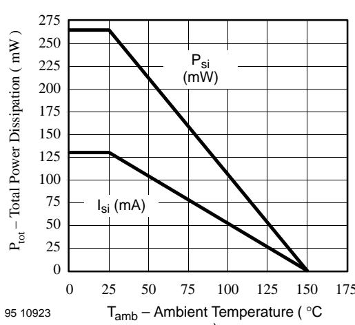
Figure 1. Derating diagram
