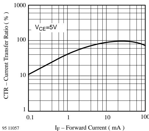
Figure 15. Current Transfer Ratio vs. Forward Current
