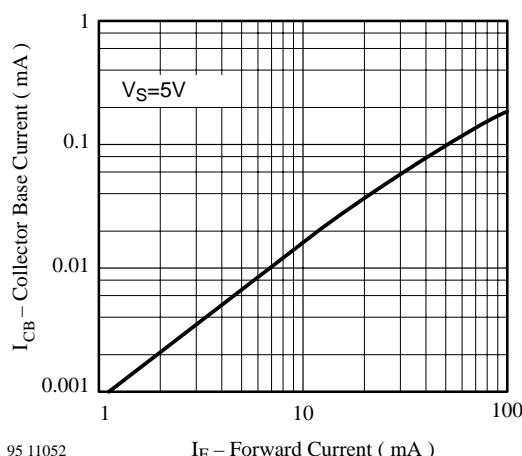
Figure 10. Collector Base Current vs. Forward Current
