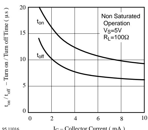
Figure 17. Turn on / off Time vs. Collector Current
