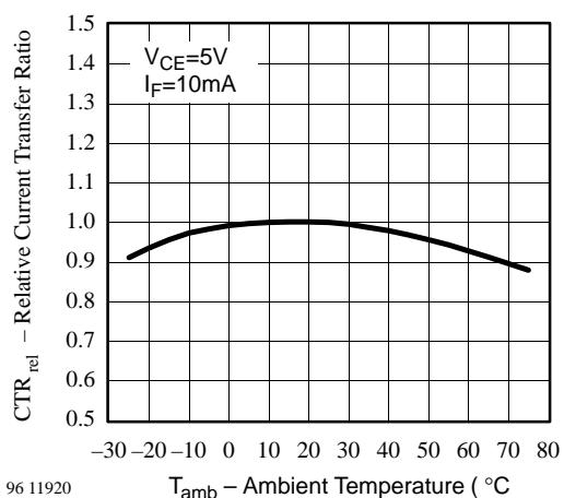
Figure 8. Relative Current Transfer Ratio vs.
