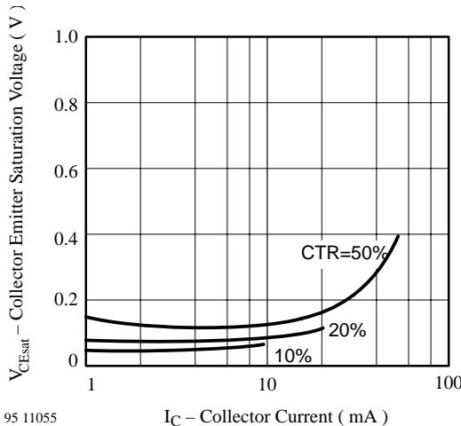
Figure 13. Collector Emitter Saturation Voltage vs. Collector Current
