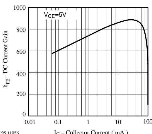
Figure 14. DC Current Gain vs. Collector Current
