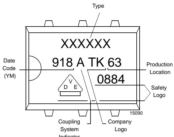
Figure 18. Marking example
