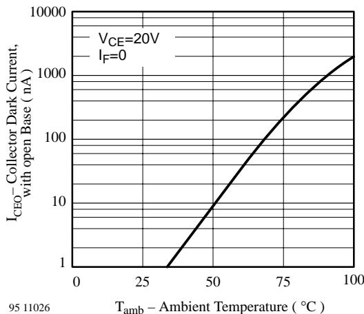
Figure 9. Collector Dark Current vs.
