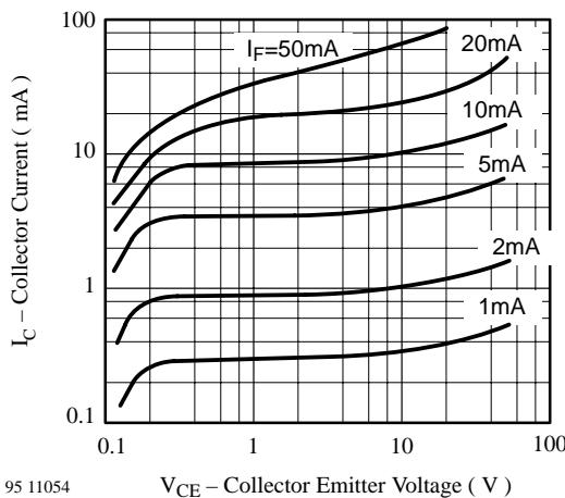
Figure 12. Collector Current vs. Collector Emitter Voltage
