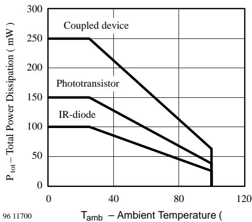
Figure 6. Total Power Dissipation vs.
