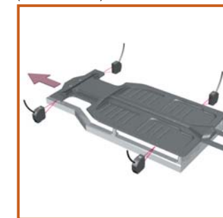
Measuring Car Body Widths (ZS-HLDS10)
