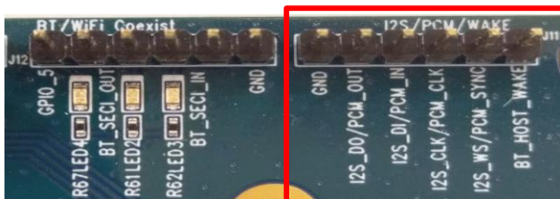
Figure 5: Pin header J11
