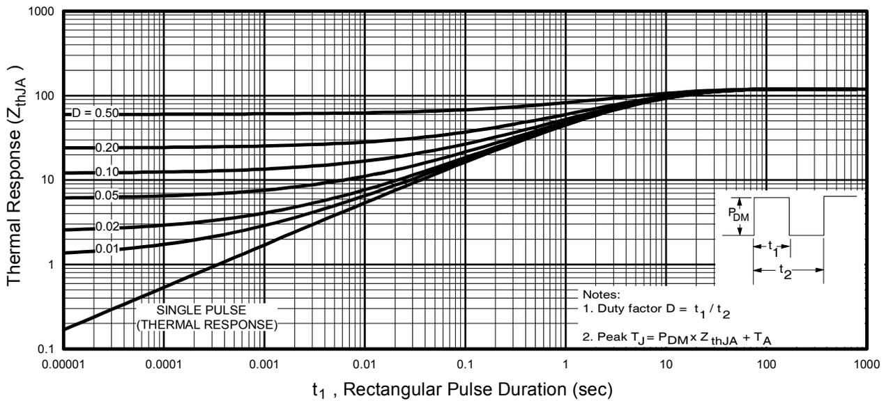
**Fig 11. Maximum Effective Transient Thermal Impedance, Junction-to-Ambient**
